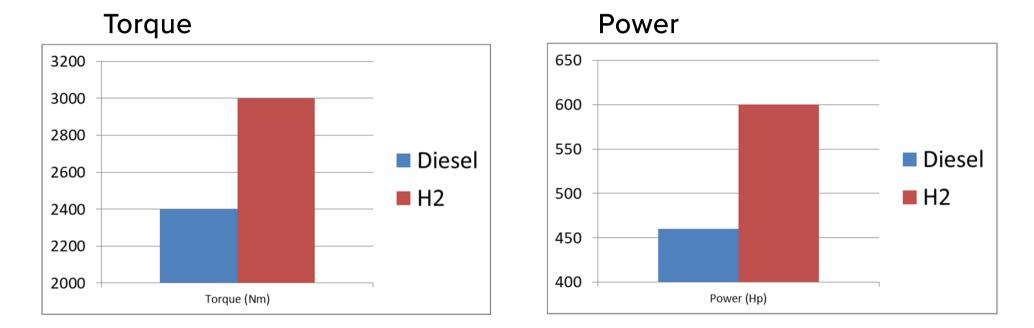
Torque and power comparison of 13-liter engine with diesel and with H<sub>2</sub> HPDI (engine limitations like PCP, exhaust temp, and boost pressure kept below limit)
