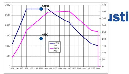
Torque Curve of Base Diesel Engine and Simulated Points
