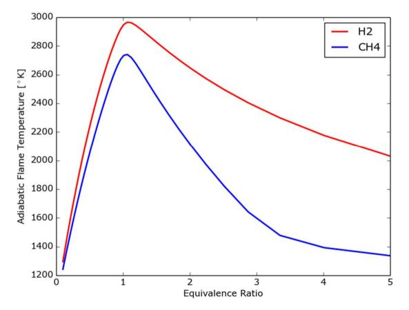
For methane on the fuel-rich side, the AFT decreases much faster compared to hydrogen. This is due to the fact that several reaction mechanisms such as the steam-methane reforming reaction and pyrolysis reactions are strongly endothermic.
