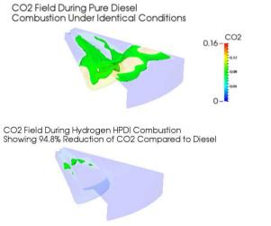
CO2 Mass Fraction of Diesel (Above) and H2 HPDI (Below)
